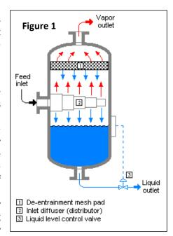
most difficult and challenging contaminants in any gas stream are aerosols. These are finely divided liquid particles with diameters ranging from a few hundred microns to less than 0.1 microns. Most of the approaches to separating liquid contamination from gas streams using demisters with mesh pads, vain packs or horizontal filter-separators have approximately 40-50% effectiveness at removing liquid aerosols.
