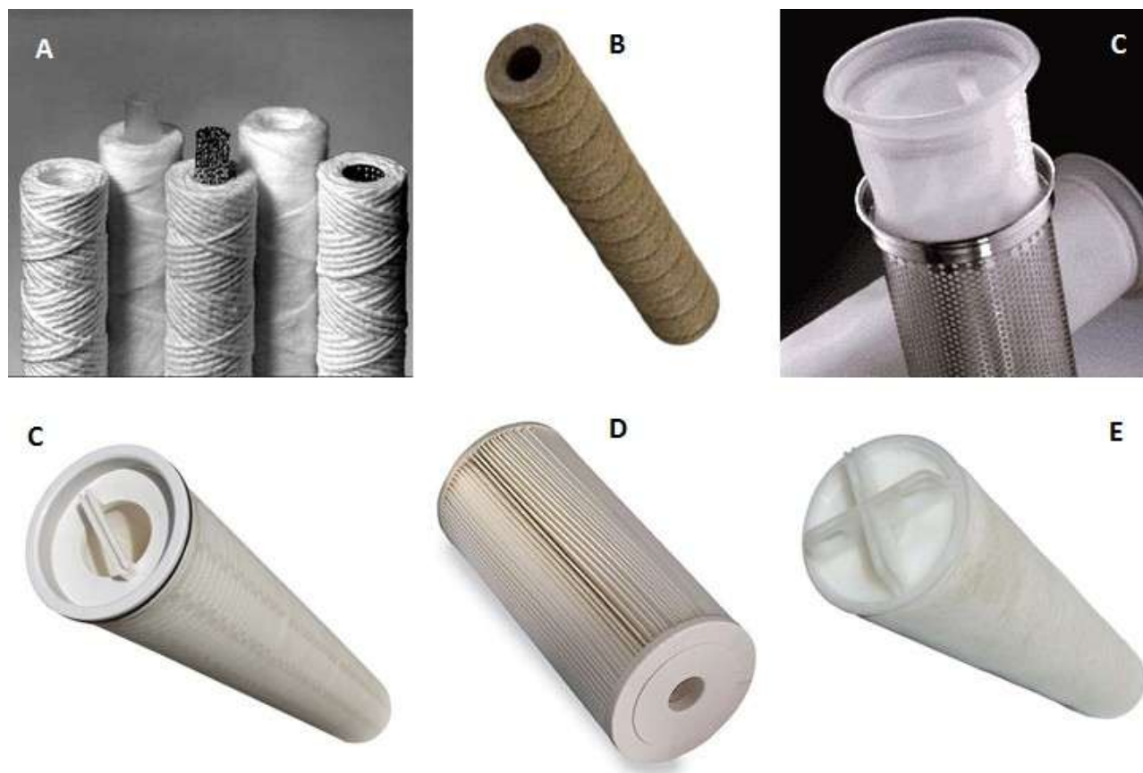
Figure 1. Common disposable cartridge amine unit filter types: A) String Wound (out-to-in flow); B) Resin Bonded (out-to-in flow); C) Bag (in-to-out flow); D) High Flow (in-to-out flow); E) Pleated Filters (out-to-in flow) and E) Axial or Radial Pleat 740 Design (out-to-in flow)
